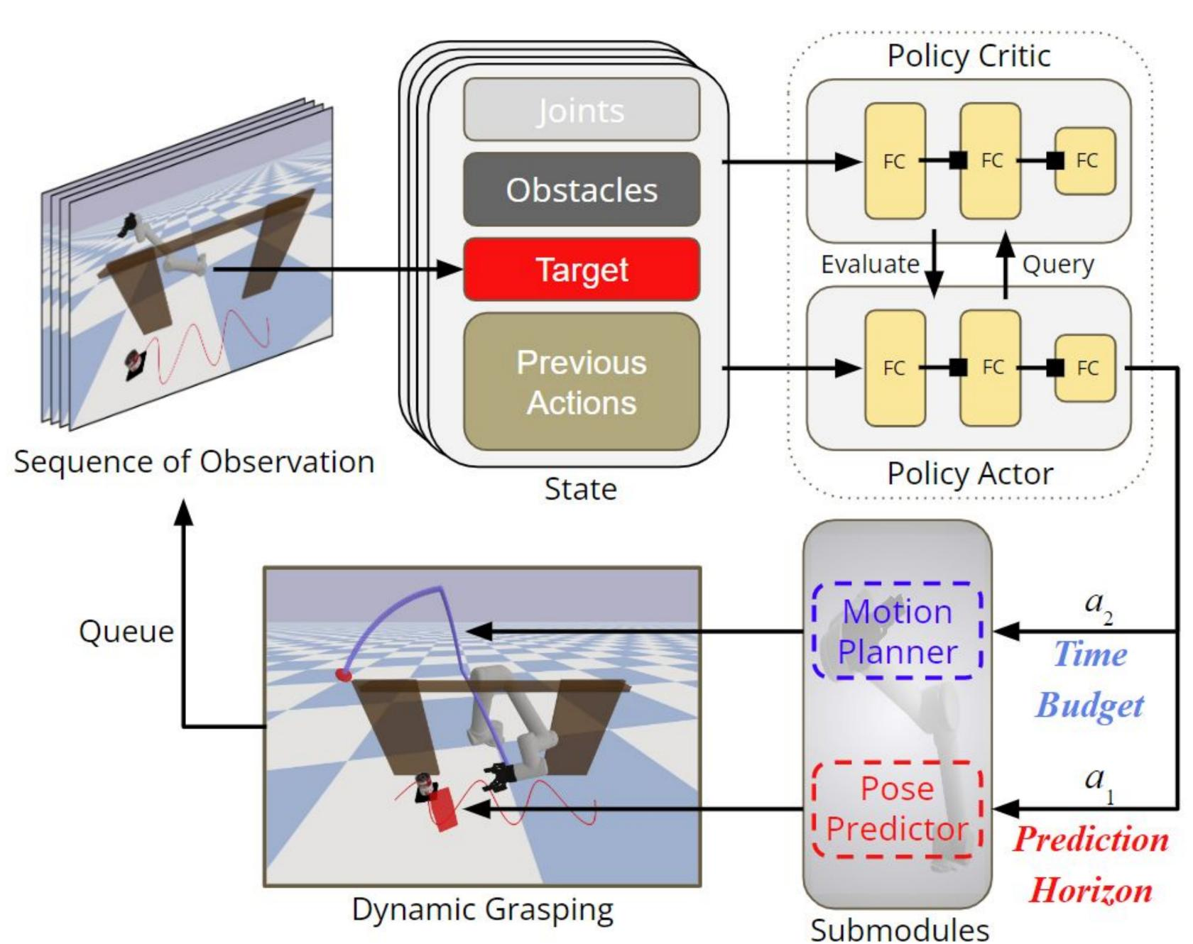
In this work, we learn a meta-controller through reinforcement learning to control the prediction horizon and time budget dynamically at each time step. Our meta-controller is trained with PPO and a sparse reward when the object is successfully picked up.
